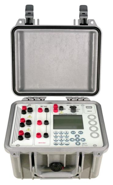
CheckSource 2.3 is a three-phase current source for currents up to 6 A. The test currents will be generated with the same frequency and a user-defined phase shift to the voltages applied to the voltage inputs. Alternatively the test currents can also be generated with a user-defined frequency.
